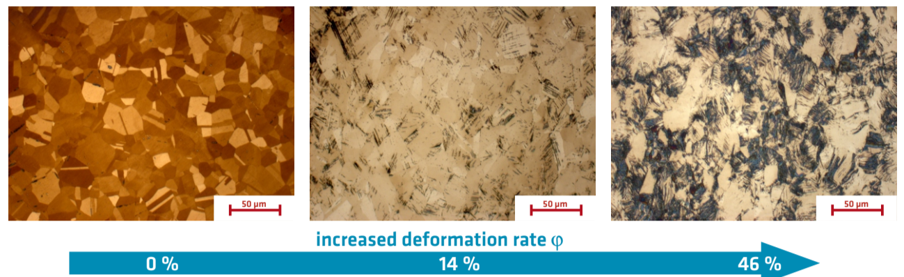
fig. 1: microstructure of stainless steel AISI 304 with different cold deformation rates, etched with Beraha I
